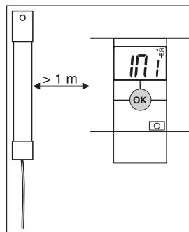
Antenna should not be located too close to the room unit during initiation.
