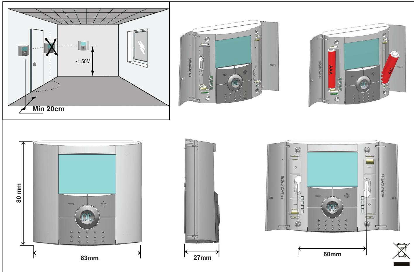
**NOTE!** We recommend that you install the room sensor using the enclosed screws and plugs, as incorrect positioning of the sensor may jeopardize heating comfort.
