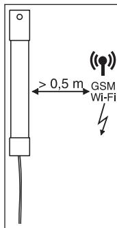
Antenna should not be located too close to other wireless units or power cables.
