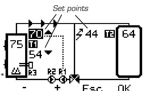
To change a set point, press OK so the value is marked with a black box (see picture on right). Use the +/- buttons to change the value and press OK to save.
